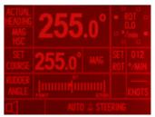
Track Mode operation provides single or multi waypoint steering performance based on data received from a proprietary ECDIS/Plotter including - when used in conjunction with an Approved ECDIS - remotely instructed constant radius turns etc.
